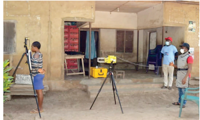
Screening of a community member with an artificial intelligence-enabled mobile X-ray device
